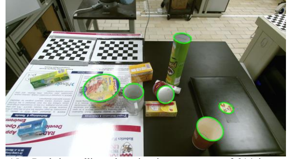
Fig. 15. Real-time ellipse detection in a sequence of 214 images. A cluttered background with light and dark colors is used to verify the robustness of the presented detector.
