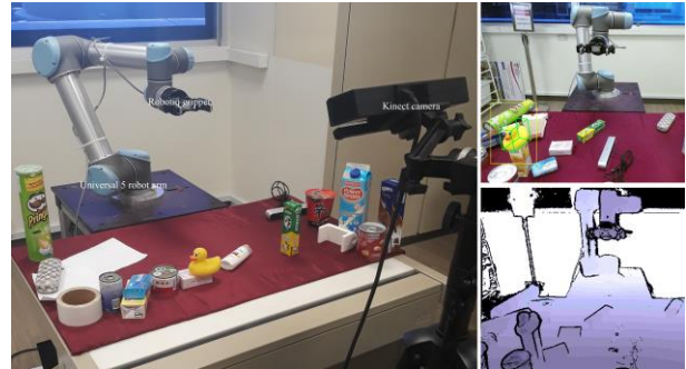
Fig. 1. Pose estimation of an object in a cluttered environment. The result of pose estimation is visualized by the green bounding box.
